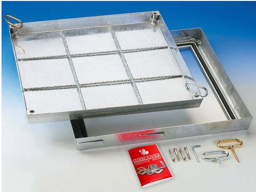
Type SBVS-250 The bottom of the cover is reinforced with IPE-beam section and flat steel
