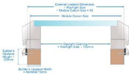
**Open Rooflight Span**
